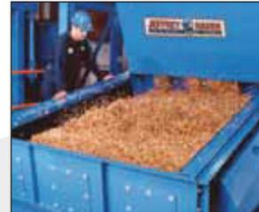
Screen decks are easily replaced and there is a wide variety of deck opening sizes and geometry available. Optional features include adjustable inclination and variable wave frequency.
