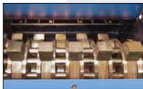
a principal similar to a wood hog, but with special features which offer a “soft touch” to the chips to minimize the creation of pins and fines. This, along with other patented components, permits it to reduce oversize chips at unheard of efficiencies, plus offer the following advantages:
