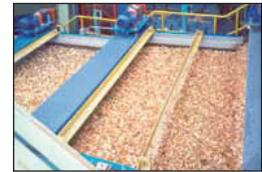
The spaces or slots between the bars are accurately pre-set and locked in place to establish the open area through which material will pass. When activated, the eccentricity of the shafts causes the bar to alternately rise and fall in a circular pattern.
