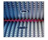
are aligned so that the pyramid apexes on one roll travel in the valleys of the apexes on the adjacent roll.
