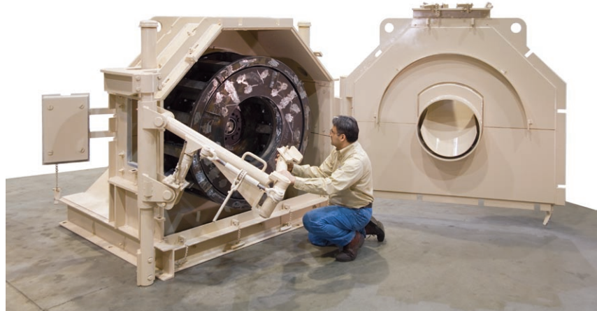
Figure 5. The Cage-Paktor cage mill has an onboard jack that swings into position to remove cages for repair without the need of overhead cranes or extra help.
