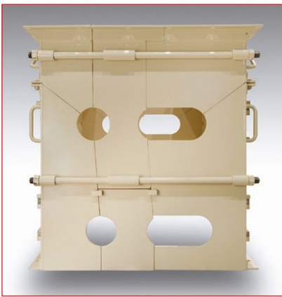
Figure 2. Roll crusher housing splits into sections for easy roll removal and maintenance.
