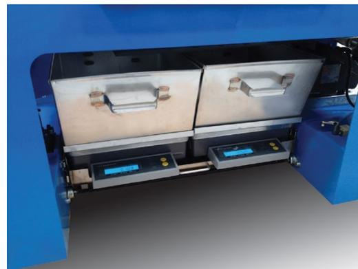
Automatic scale weigh bins ensure easy access to samples
