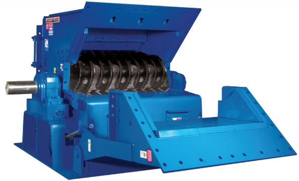
unique to our hammermills. Unlike conventional screen sections, the Slant-Flow design is angled into the flow of the material being shredded. This provides more shredding action and allows the material to evacuate faster. The result is less wear on the grates and hammers, and a more uniform product size.
