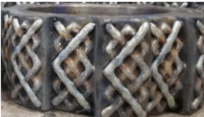
Duralife® XP ring and paddle hammers with advanced alloys and hardfacing
