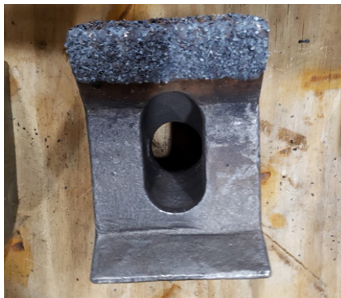
Ultralloy® XP solid hammers and replaceable tips with advanced alloys and hardfacing
