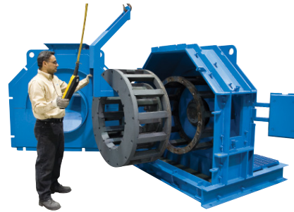
Swing-away door on Model 50 speeds maintenance.
