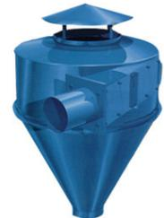
Replaceable and rotatable cone liners and R-35 (600 BNH) cast inlet segments are available as options. R-35 is extremely wear resistant and ideal for abrasive applications. Ceramic liners are also available.
