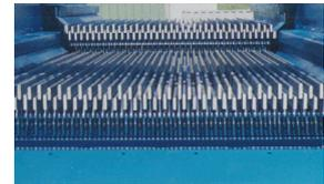
The spaces or slots between the bars are accurately pre-set and locked in place to establish the open area through which material will pass. When activated, the eccentricity of the shafts causes the bar to alternately rise and fall in a circular pattern.
