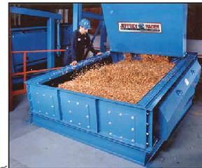
Our **CC2000** allows mills to classify chips according to user-defined thickness. Features include:
