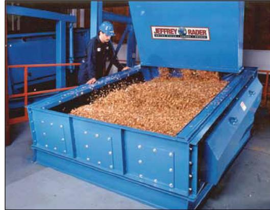
particles. In addition, the alternating wave motion slightly varies the perforation geometry, either accepting or rejecting near-size particles. When combined with the forces of high acceleration, blinding is eliminated. This self-cleaning feature is particularly beneficial in harsh climates where screen blinding or plugging has always been a problem.
