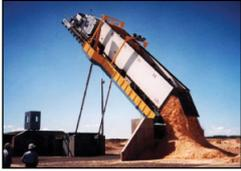
Permanent truck dumpers are available in drive-through, back-on and extended arm configurations for both grade-level and elevated
