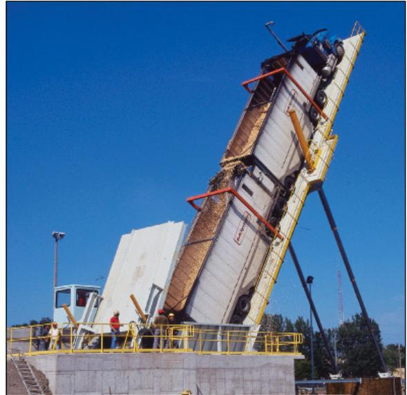
solenoid-operated from the panel. Limit switches at various system points ensure the proper operating sequence. The simplified controls permit efficient operation from a single, remote-control station and/or by the driver alone.
