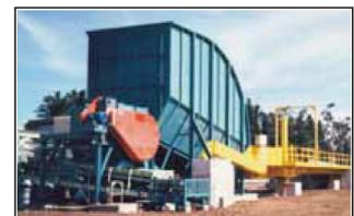
Chain, auger or stoker discharge systems built into the hoppers meter materials evenly from dumping to storage to processing.
