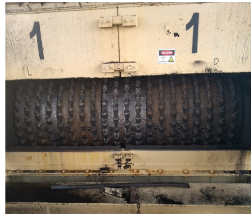
Abrasion-resistant advanced carbide rolls installed in customer site
