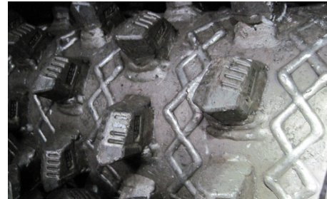
Partial hardfacing in "X" pattern with Duralife tooth
