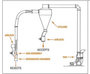
Each ADS system is custom tailored to accommodate your specific process requirement resulting in the elimination of unnecessary energy consumption.
