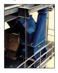
Our Air Density System is then used to remove knots, dense fiber, metal and rocks from the reject flow prior to the chips going to the over-thick processor.
