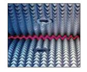
pyramid apexes on one roll travel in the valleys of the apexes on the adjacent roll.
