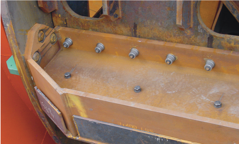
Figure 1. A close-up view of huck bolts on a Mega Breaker. Huck bolts are an option on all Bradford Breakers.
