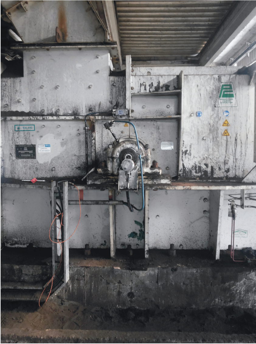
Figure 3. A Pennsylvania Crusher TKK granulator after more than four years of consistent and reliable service.
