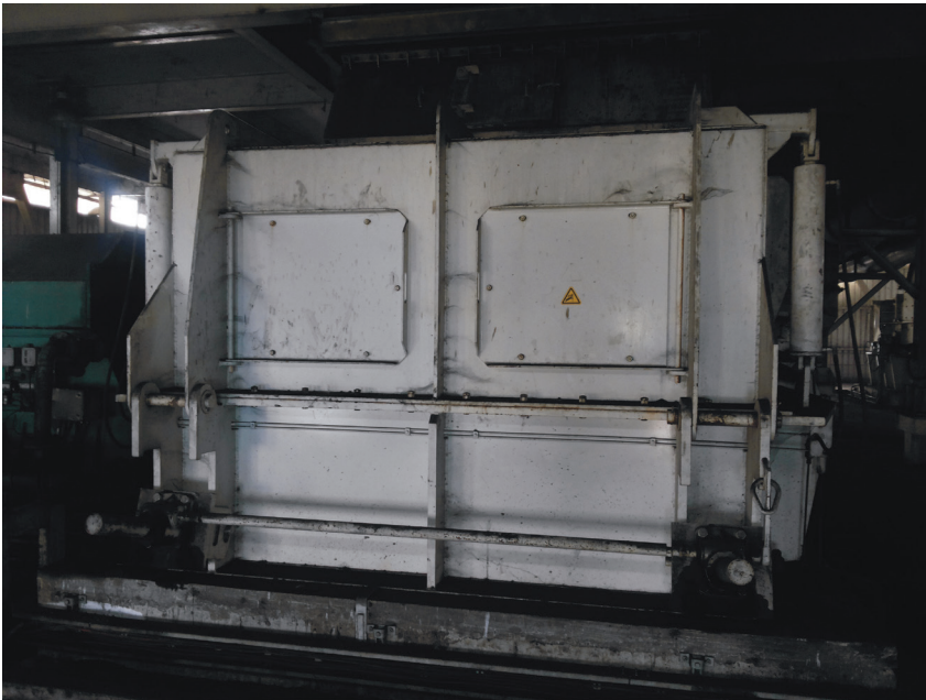
Figure 2. Clean-out doors on the granulator offer easy access to clean out the tramp iron pocket.
