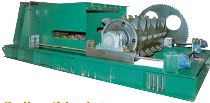
Typical Frozen Coal Cracker installation under a rotary car dump or reclaim hopper.
