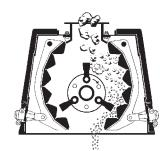
The reversible impactor is a highly versatile crusher first developed and patented by Pennsylvania Crusher in 1937.
