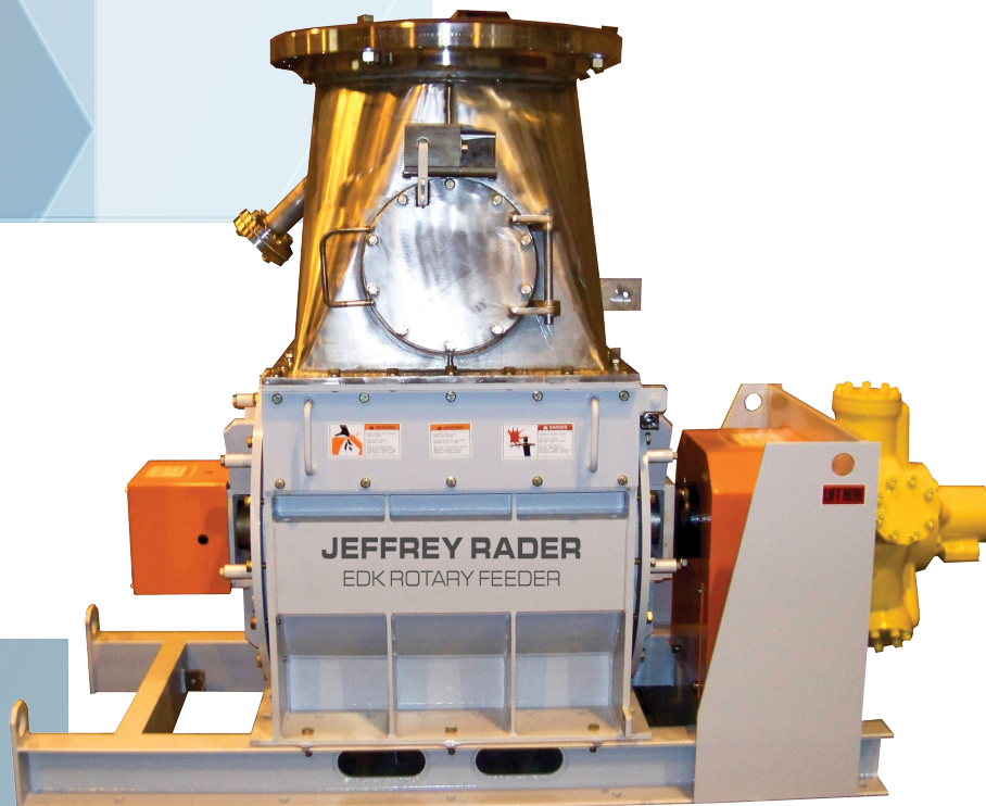
EDK Rotary Feeder/Delumper (25 x 30) with Optional Stainless-Steel Transition
