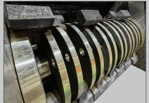
Suspension discs are keyed to the shaft.
