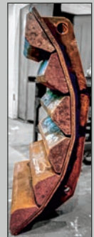
Curved breaker block assembly matches the hammer arc.
