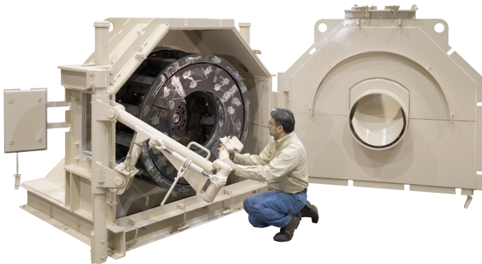
Optional cage jack is available on 2C4R to aid in cage removal.
